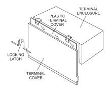
Figure 12. Plastic Face Plate (UVWO Terminals)
